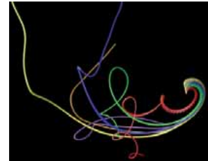
Figure 1: Particles with different inertia, as they evolve after being released from within a small scale vortex filament. A Lagrangian tracer (red) is strongly sensitive to small scale vortices from the advecting turbulent flow. Particles with higher and higher inertia (green, blue, yellow, etc) are less and less sensitive to small scale vorticity. For a relatively small Stokes value 0.16 (green trajectory) the effect of the turbulent vortex is already barely felt by the particle.
