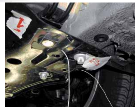
Flat microphones on the underbody of Grande Punto in the wind tunnel.
